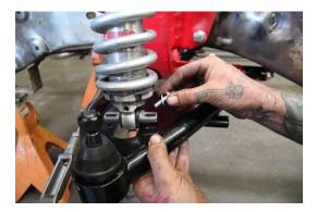
Install the coil over shocks from top to bottom but be sure to face the adjustment knob towards the outside on the top to allow for easy adjustment. Run the nut and bolt through the top mount and then move on to the bottom. The bottom arm mounting plates offers you a choice of two different mounting locations, one pair sets the shock closer to the cross member, while the other set places it towards the outside. C-10's prefer the outside mounting holes setting the geometry in proper alignment.
