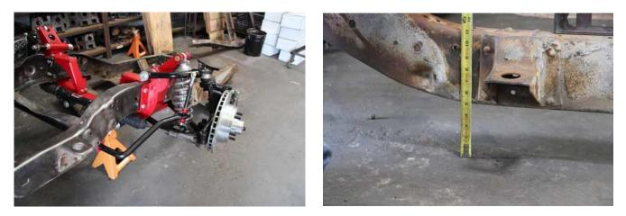
Here's a close look at the front end fully assembled before the wheels and tire were put back on. One great feature about this kit is that it allows brake clearance for wheels beginning at 15." Once we put the truck back on its wheels and had the power train in place we took a measurement of ride height clearance. We came up just 5" of frame to ground clearance!
