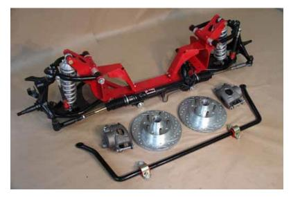
Shown here in the photo is the complete Wide Ride front suspension system for the '63-'72 GM C-10 truck line. As mentioned before, this unique set up is a true "bolt on" system that does not require any cutting or welding. The system can also be purchased at different levels while remaining operational.
