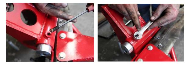
The cross shafts are held in adjustment by two set screws. Before you install them in the cross member place a dab of "anti-seize paste" on the threads and sung them down. To ensure that the set screws stay tight, a lock nut snugs them down tight.
