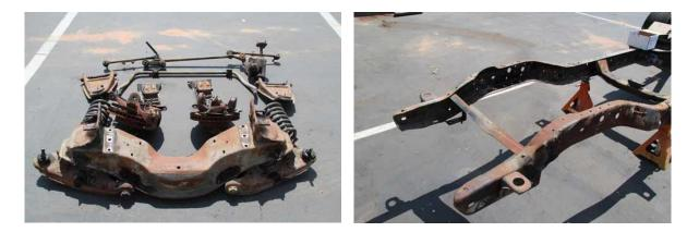
This '71 Chevy C-10 (the cab and engine were removed for photo purposes) was really chosen to lose its factory front end and all the headaches that go along with it. We wasted no time tearing into the truck at No Limit. We removed the entire front suspension, steering, and brakes using nothing more than some hand tools and rust penetrate in just under an hour.
