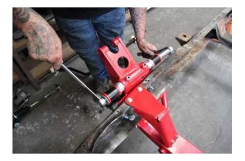
To install the upper arm, align it with the cross shaft hole and slide the long fastener through the arm and the shaft. Be sure to use the supplied washer in between the "A"-arm bushing and the cross shaft to maintain the bushings integrity. Finish it off by installing the nuts on the shafts fasteners and tighten them down tight while allowing the arm to travel up and down with some resistance.
