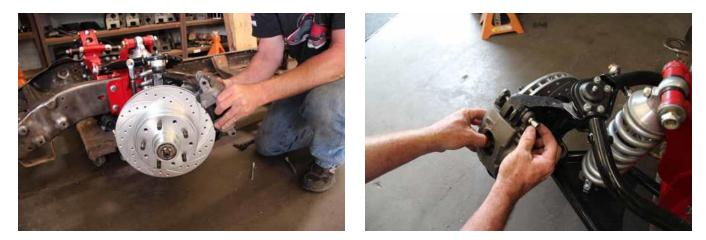
The method to installing the calipers is just like factory GM specs, as the pads stay in place between the rotor as the caliper surrounds it. To fasten them slide the pins through the caliper and spindle and snug them down.
