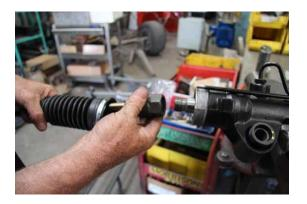
To install the extension you'll need to remove the clamps that hold the tie rod dust boot in place. Next, using an adjustable wrench, break loose the inner tie rod at the knuckle joint and spin it free.
