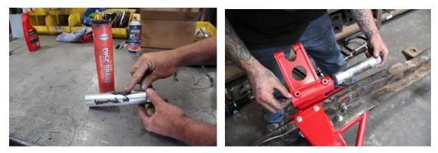
The upper cross shafts that hold the upper "A"-arm are made from solid billet aluminum and need to be greased before installing it into the cross member.
