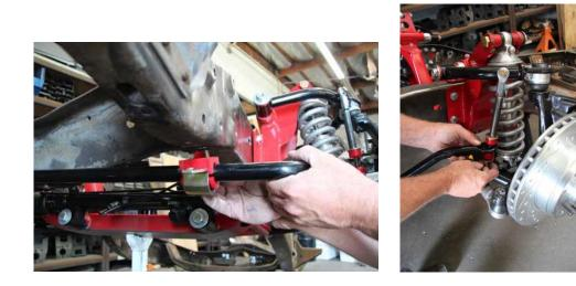
Run the fasteners through the frame and the "frame to bar" mounts. Next run the bar's "links" from the eyelet on the bar to the upper control arm. Leave these fasteners loose until the truck is back on the ground under weight, and then snug everything down.
