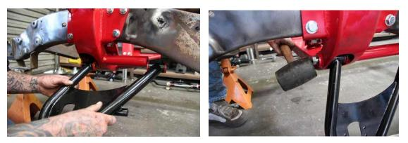
The front mount of the bottom "A"-arm lines up with a pocket in the cross member while the rear tucks behind the stub of the cross member. Once in place, slide the long bolt through the cross member and the "A"-arm using a rubber mallet for persuasion.
