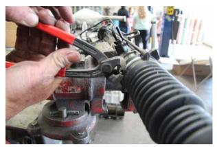
Use thread locker before installing the extension. After you install the extension repeat the process of using thread locker on the extension before re –installing the inner tie rod knuckle. Now re-install the dust boot and clamp the band back down to the rack body so that the boot stays in place.
