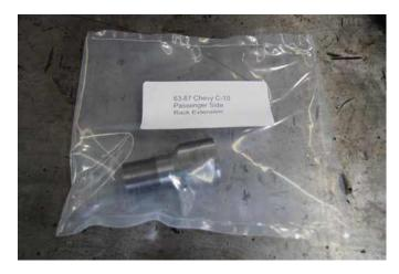
Supplied in the kit is an inner tie rod extension for the passenger side of the rack and pinion.
