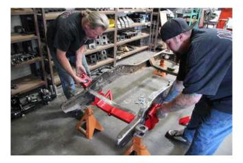
Place the frame on a set of jack stands and check to see if the frame is level. Position the jack stands where they won't interfere with the cross member location. Next, grab a buddy to help slide the cross member under the frame rails and up into the stock frame rail mounting holes. The best way to accomplish this is to move the cross member forward first towards the steering box mounting holes, then swing it back while lifting up towards the rear.
