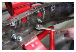
Align the holes from the stock cross member with the holes on the bottom of the Wide Ride cross member and run in the supplied fasteners. Do the same on the side plates located on the outside of the frame rails, which might need to be opened up with the assistance of a ½ drill bit and a drill motor depending on the model year of your trucks frame. Finally, snug the bolts down tight using a cross pattern to keep things square.
