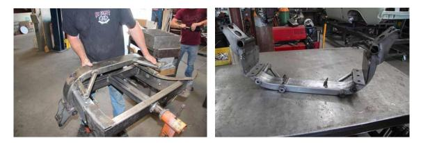
Here's a peak on how each cross member is assembled in No Limit's "frame jig" purposely built for the C-10 Models. This is a good look at the raw cross member straight out of the jig fully welded and ready for shipment.
