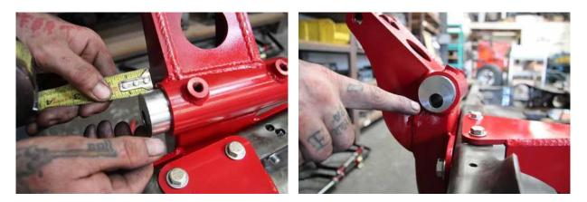
Slide the cross shaft in place from the rear while allowing 5/8 of an inch to protrude out of the cross member. Also note that the cross shaft mounting hole is drilled off center, creating an eccentric bushing to allow for camber adjustments. The best place to start is to line it up in the six o'clock position during the install.
