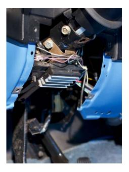
The next item to remove is more involved. You must remove the steering column from the truck. We have tried to install these with it just dropped down and it will not work. The first step will be to disconnect the steering intermediate shaft from the column output (in the engine bay) as well as the column clamp fasteners, and the shift linkage if you have a column shift column.
