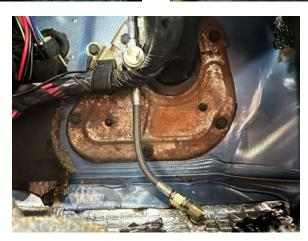
Refer to the photos above for final pressure hose installation. Measure over 2" from the bottom bolt in the lower column seal and down 1.75" from the edge of the toe board. Mark this location and install the pressure bulkhead fitting. You can now final tighten all of the pressure hose connections and reassemble the truck.
