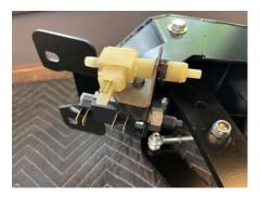
**Step 4** - At this time you can go ahead and install the new pedal assembly. Put the studs through the firewall first, then lift it straight up toward the front of the dash. You can temporarily install the bolt for the column to help the pedal assembly up. (Note: we have installed these into a few cabs and have found that there is a big difference in how they fit the dash. Please see the photo below.)
