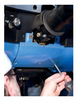
Once the cover is off, you will see the driver side vent vent and the wiper module (81-87). Remove the crossover duct as well as the wiper module that is attached to the column.
