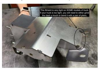
**Step 5** - It is now time to do the plumbing and the first step is to mount the reservoir out in the engine bay. We have supplied you with a mounting bracket that locates the reservoir utilizing the windshield wiper mounting holes. We suggest installing the reservoir first, then determine the bulkhead fitting hole location by using the hose attached to the reservoir. I would also just drill an 1/8" pilot hole for now.
